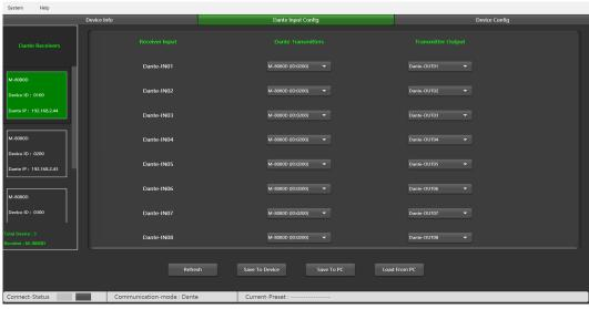
The Dante-IN01 of the M-8080D (ID:0100) receives audio signals from the Dante-OUT01 of the M-8080D (ID:0200).
