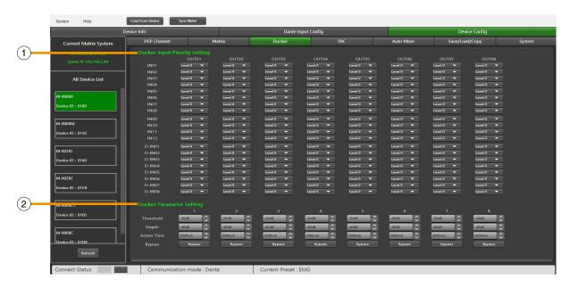
The principle of the Ducker is to attenuate one or several channels when priority signals are activated.
