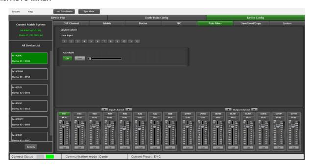
The Auto mixer automatically controls the gains of multiple microphones in real time, dramatically reducing feedback, noise and comb-filtering from adjacent microphones. It maintains a consistent system gain, even when multiple speakers are talking simultaneously, and makes perfectly matched crossfades, without any signal compression.
