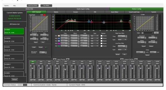
Adjusting the high-pass filter to 32.7Hz. Type is adjusted to BW24. Drag EQ1 to 54.4Hz and adjust the Q value to 2.0. Gain up to 8dB. Drag EQ2 to 315Hz. Q value is adjusted to 2.5. Gain to 2.5dB. EQ3 type to 1.45kHz The Q value is unchanged. The gain is attenuated to -2.5dB. The EQ4 type is adjusted to 406.1Hz. The Q value / gain is unchanged, and the EQ5 type is adjusted to 8.38KHz. The Q value does not change and the gain reaches 4dB.
