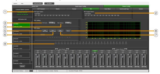
FBC (Feedback compression) function can effectively suppress howling expansion volume, ensure voice transmission quality, high fidelity, and clear sound.
